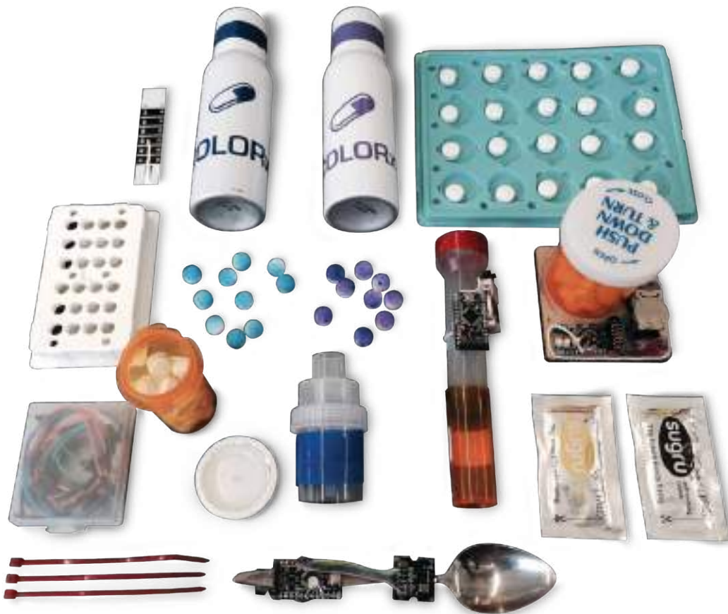
▲ The medication adherence kit includes an array of accessories to do tasks such as monitor medication usage and weigh pill bottles. It includes ergonomic tools such as simple zip ties to adjust the grip and hold of medication containers. Color-coded pills can be produced by spraying food grade coatings to differentiate medications.
