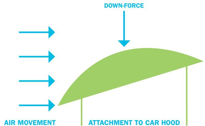
Notice how the air moves. The air strikes the front of the airfoil, which is slanted down. The angle of the air against the foil causes a push, or force, downward. The airfoil is attached to the hood and therefore forces the car downward onto the track, allowing greater traction for cornering (see Fig. 4).
