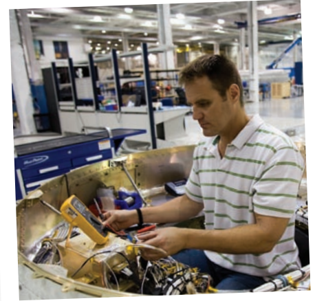
Test and installation of rocket electrical circuitry.
