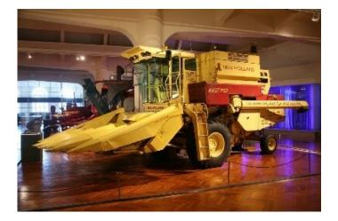
**1975 New Holland Combine:** Combines are named this because they combine the three jobs of picking ripe grain - cutting the stalks off in the field; removing the kernel of wheat, rye, or corn from the plant; and separating the kernels from the straw or stalks. Combines save lots of time and only need one person to drive them. It is called self-propelled because it does not need to be pulled by another engine.
